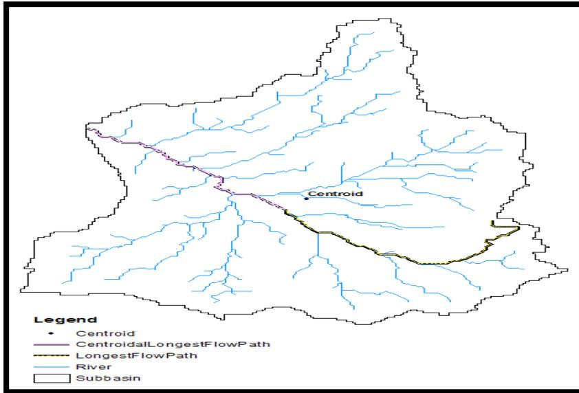
Figure 3. Güvenç Basin physical characteristics generated with HEC-GeoHMS.
